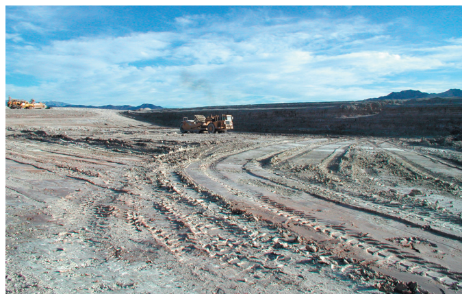
Figure 4. Belly dump mining of overburden in an IMV Nevada sepiolite pit; overburden in this area is about 5 m thick.
