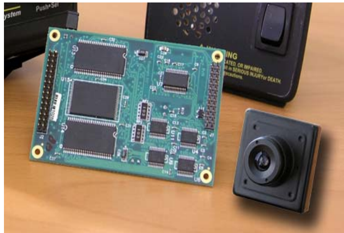
Figure 16. Forward-looking LDW camera system hardware
