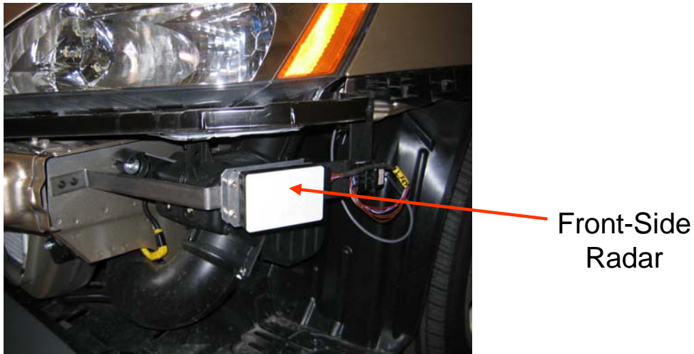
Figure 25. LCM short-range radar sensors
