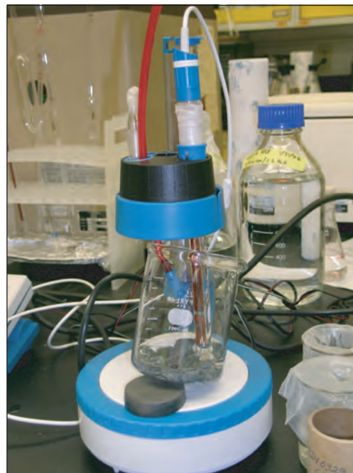
Figure 3. Laboratory ANC test apparatus. Glass beaker contains water and rock fragments (gray). Acid is added to the sample through the red tube; probe (center of beaker) monitors pH.
