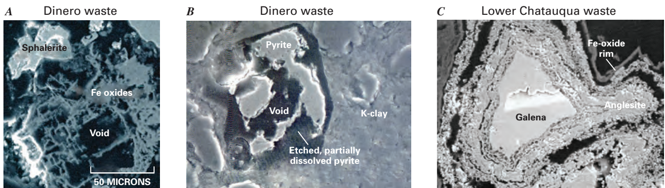
Figure 2. Trace-element-rich sulfide minerals commonly show partial to total dissolution in mine-waste piles. (A) Sphalerite ( [Zn,Fe]S ) shows partial dissolution and remnant iron-oxide rims. (B) Pyrite ( FeS ) is deeply embayed and etched by dissolution processes. (C) Galena ( PbS ) has partially altered to anglesite ( PbSO_4 ). Fine-grained, porous anglesite rinds show partial to total dissolution, indicating that weathering of galena and the subsequent dissolution of the secondary weathering product, anglesite, is the primary source for lead in solution.
