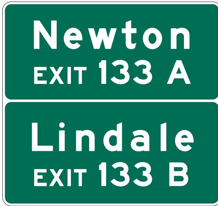
Figure 2E-17. Supplemental Guide Signs for Multi-exit Interchanges
