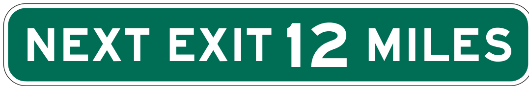
Figure 2E-16. Next Exit Supplemental Advance Guide Signs
