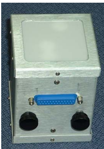
Figure 33. CROPSCAN Multispectral Radiometer (MSR). (Size is 8 X 8 X 10 cm)
