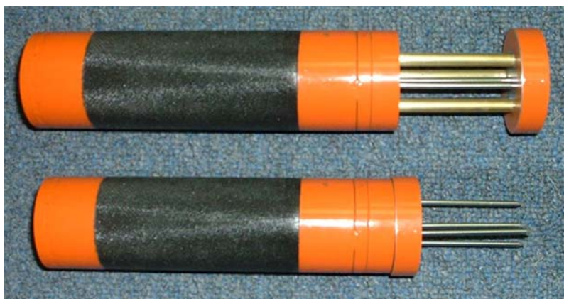
Figure 24: SMITY, Soil Moisture Insertion Tool, with slider extended and retracted.
