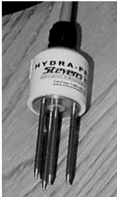
Figure 30. The Hydra probe used at the tower locations.
