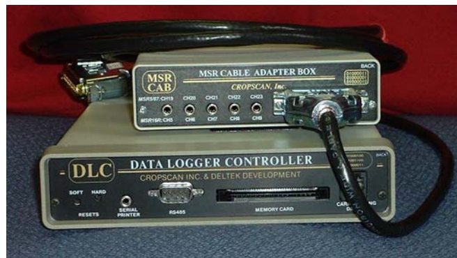
Figure 34. data logger controller & cable adapter box
