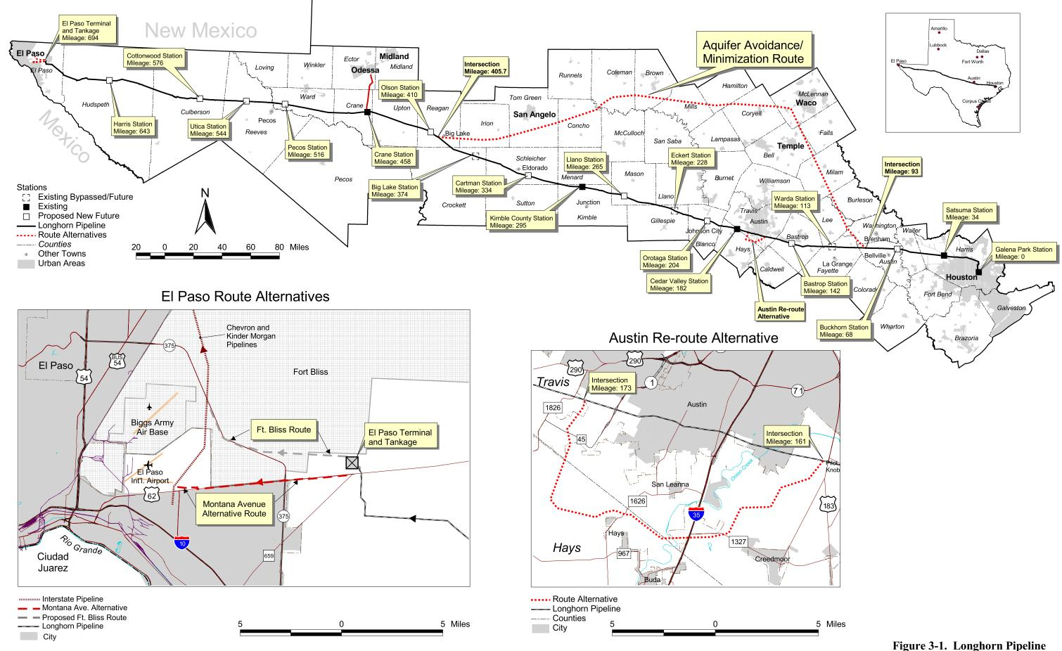
Figure 3-1. Longhorn Pipeline System and Route Alternatives
