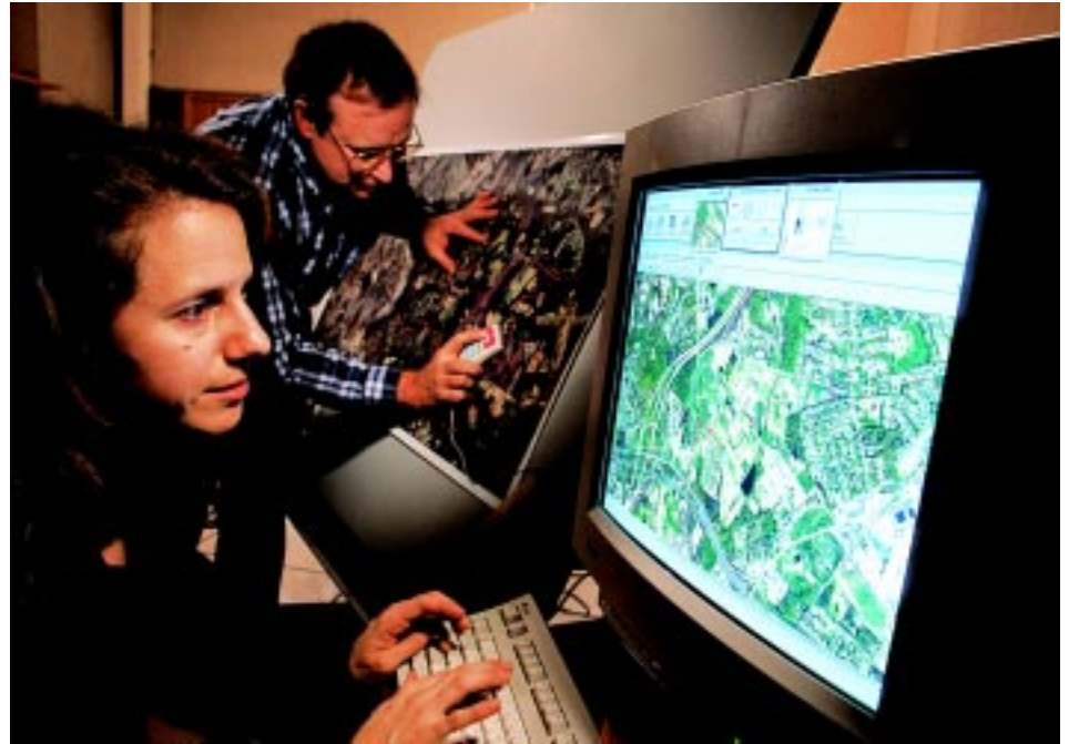
Sara Loechel, a remote sensing researcher at the University of Maryland, labels fields, woodlands, and streams on a computer, while ARS agronomist Craig Daughtry locates the same features on an aerial photograph of the Beltsville [Maryland] Agricultural Research Center. The computer image will form the base layer of a geographic information system map. Other data about soils, crops, and management practices will be added, along with remotely sensed images of crops to update their growth and development.
