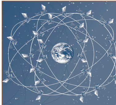
GPS uses a minimum of 24 satellites and ground receivers to track movement for navigation. (Illustrated by Norris S. Padmore)
