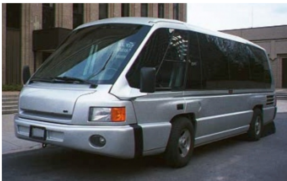
Advanced vehicles include technologies such as the Compressed Natural Gas (CNG)/electric hybrid composite bus shown here.
