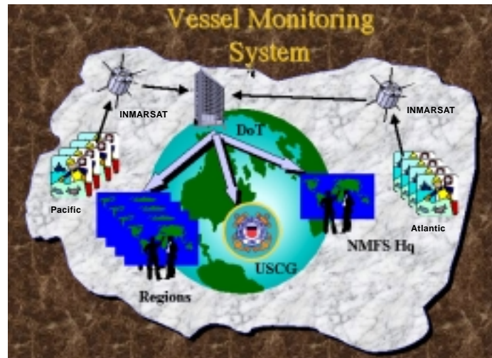
The VMS is a satellite-based tracking and communications system.
