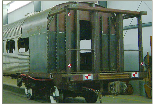
The test vehicle was a Budd Pioneer cab car retrofitted with an end structure of crash energy management design.
