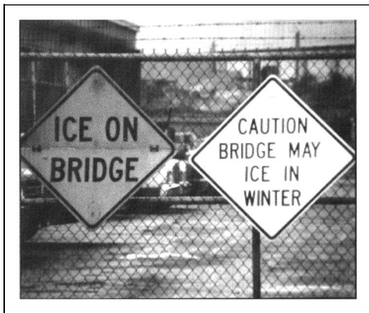
Figure 85. Warning sign with deteriorated retroreflectivity
