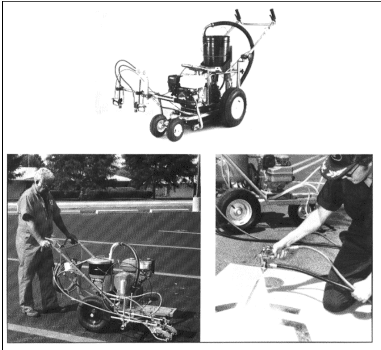
Figure 21. Small paint application units
