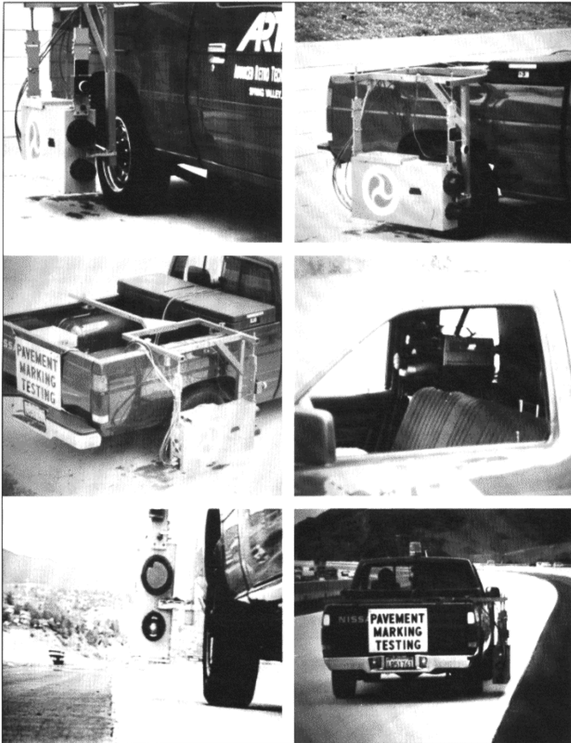
Figure 91. Pictures of the truck-mounted laser retroreflector
