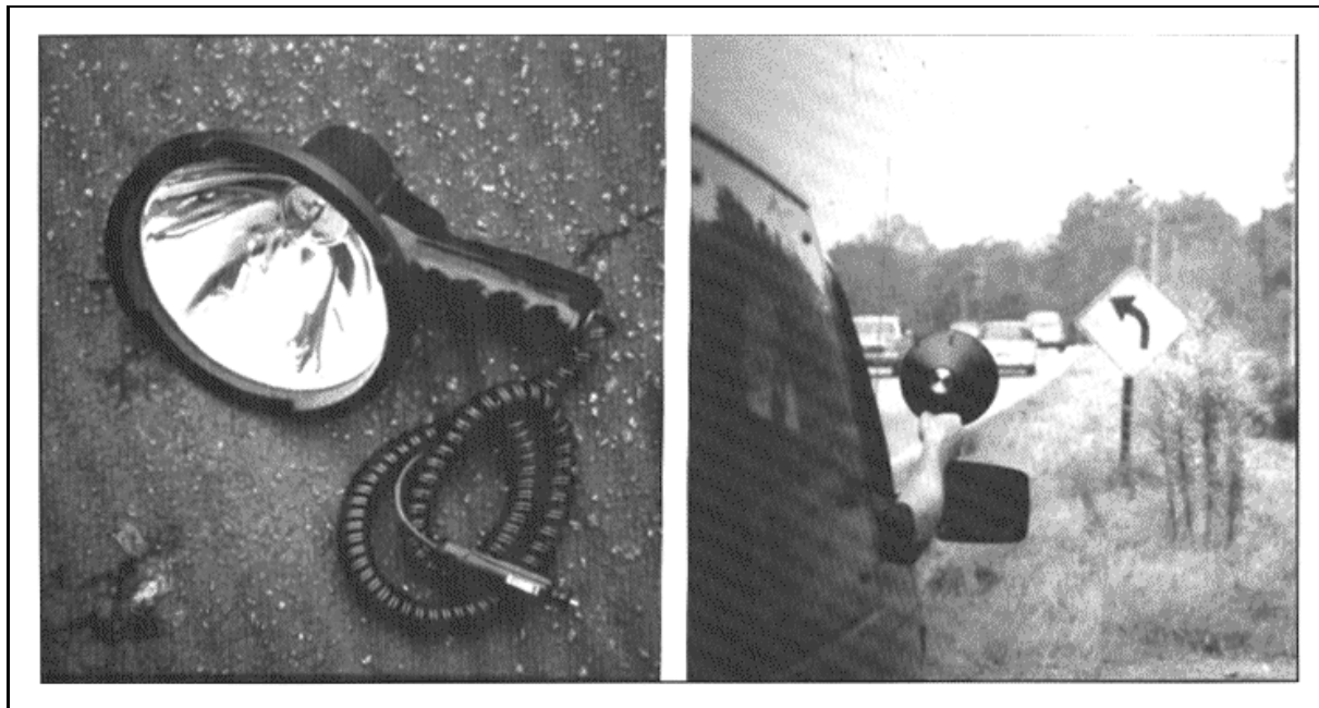
Figure 84. Daytime inspection of sign retroreflectivity
