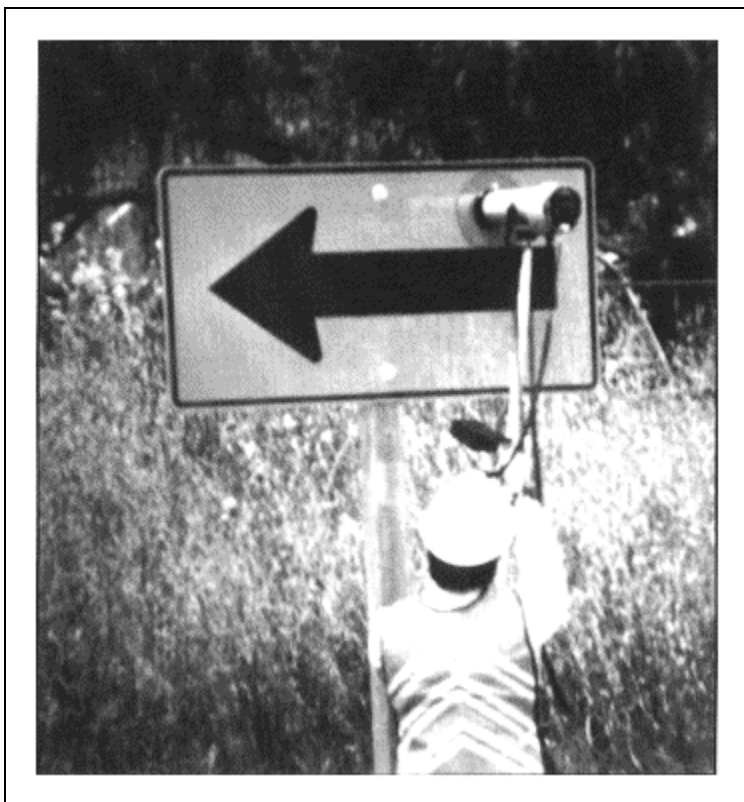
Figure 86. Use of a portable retroreflectometer
