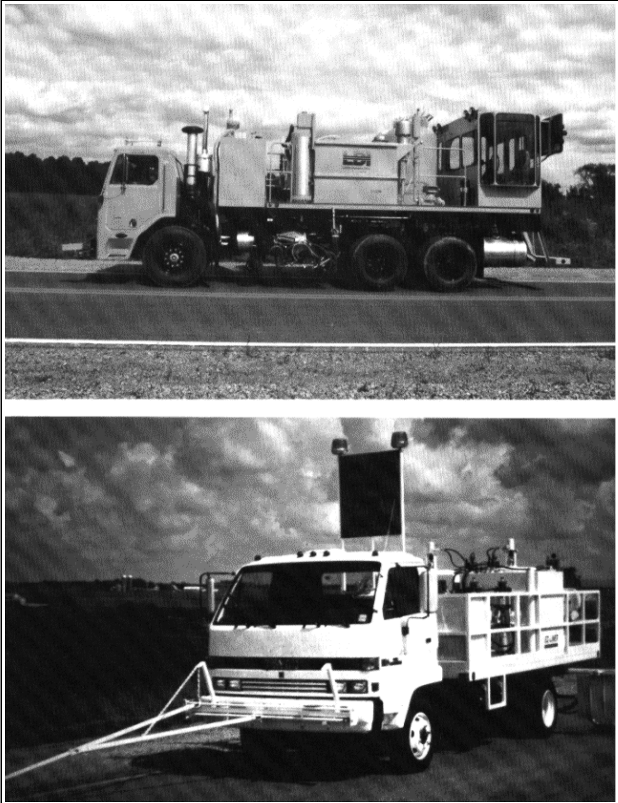
Figure 23. Truck-mounted paint application units
