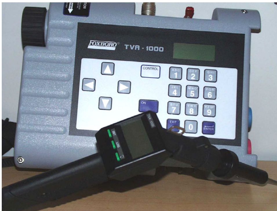
Figure A-6. Typical Federal Reference Method 21 Portable Fugitive VOC Analyzer.
