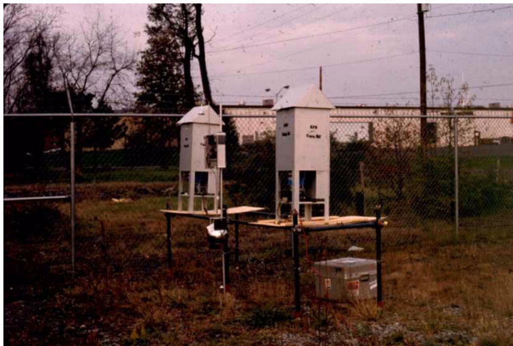
Figure A-16. Time-Integrated perimeter Air Monitoring System at a MSW Landfill.
