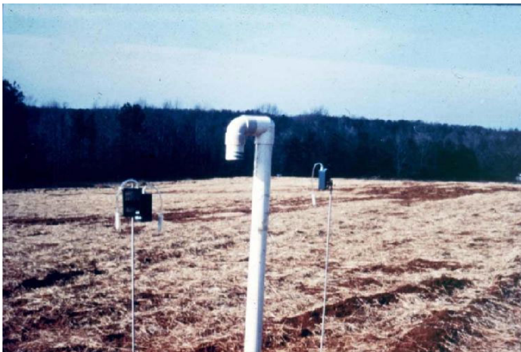
Figure A-13. Upwind/Downwind Sampling for PCBs from a Landfill Vent,
