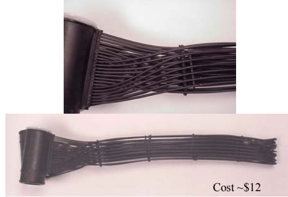
Fig. 6: Prototype low-cost polymer heat exchanger (10). Tubes are 1/8-inch (3 mm) diameter. Tube weaving and tube-to-header welding are automated processes, contributing to a low cost projection.
