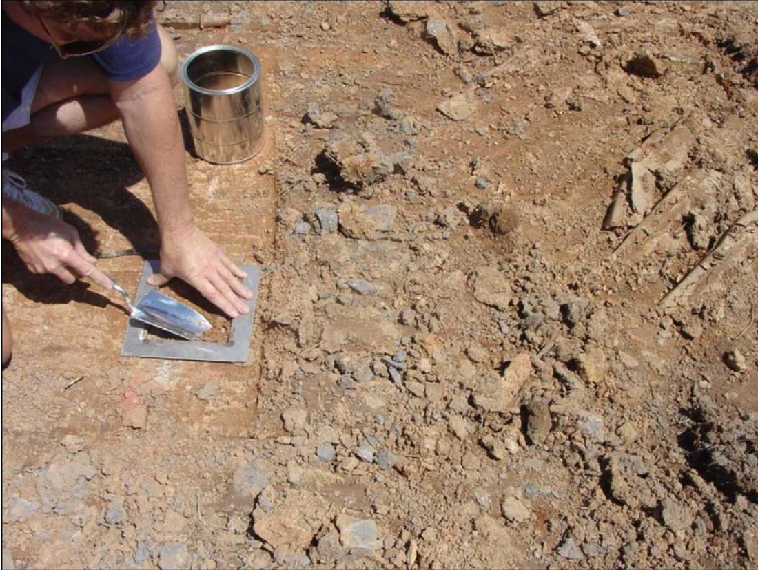
Figure 5-1. Soil sampling after the NESHAP demolition.
