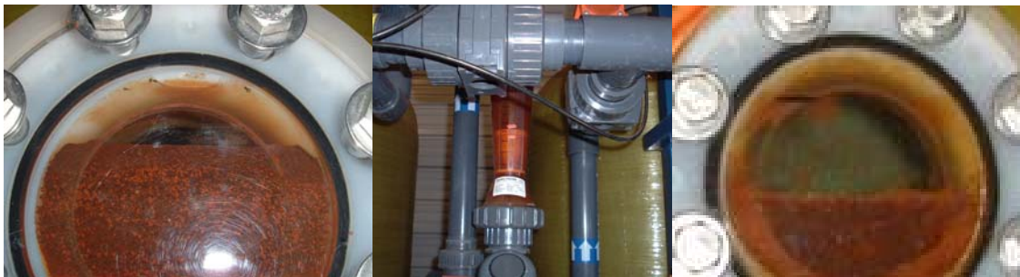
Figure 4-9. Media Run 4 Changeout Photographs (Left to Right: Initial ARM 200 Media Level through Viewglass, Backwash Water Clarity, and Media Level after Excess Media Removal)
