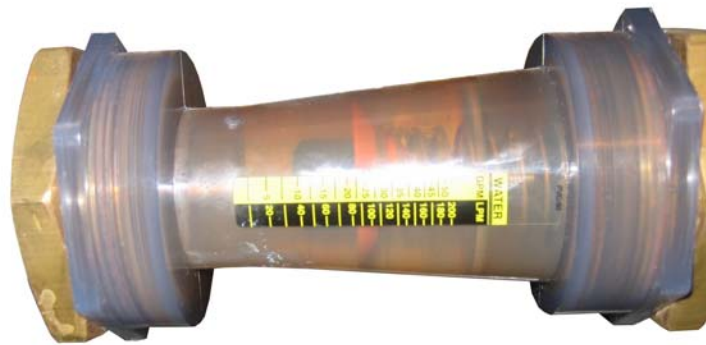
Figure 4-11. Close-up View of Insite® PX-50 GPM-12-V-F Flow Meter
