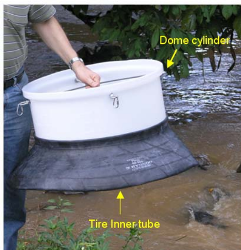
Figure 12. Tire inner tube placed around dome cylinder to improve seal to formation. Photo by Göran Bengtsson, Santo Domingo, Nicaragua.
