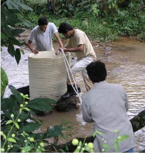
Figure 14. Open cylinder used for advective flow measurement. Photo by Göran Bengtsson, Santo Domingo, Nicaragua.
