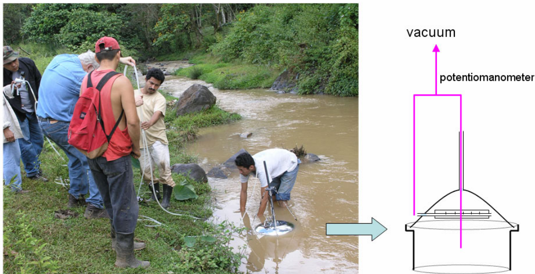
Figure 13. Bernoulli Effect is anticipated under the turbulent flow conditions in the rapid stream. The schematic illustration shows installation of potentiomanometer for head differential measurement. Photo by Göran Bengtsson, Santo Domingo, Nicaragua.
