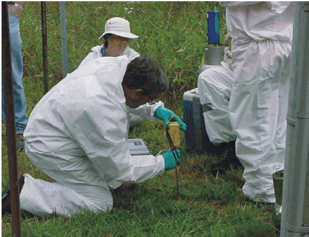
Fixed Gas Sampling Collected by Sampling Probe
