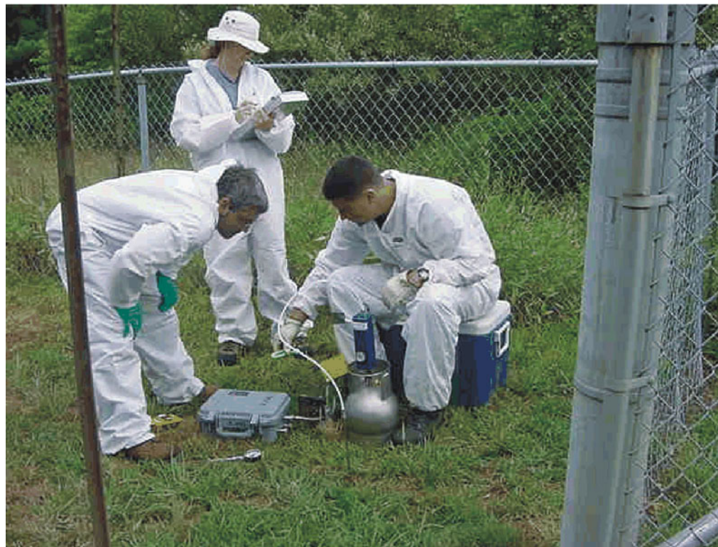
Tedlar Bag Chamber and Summa Canister Sampling
