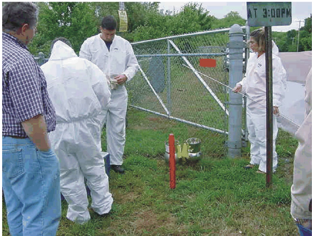
Slam-Bar Used for Sampling Probe Insertion
