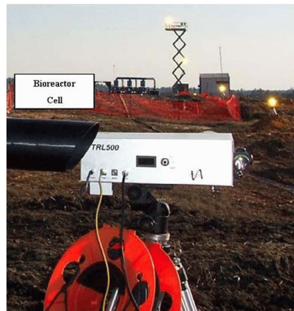
Figure 2-6. OP-TDLAS Configuration Used at the Site.
