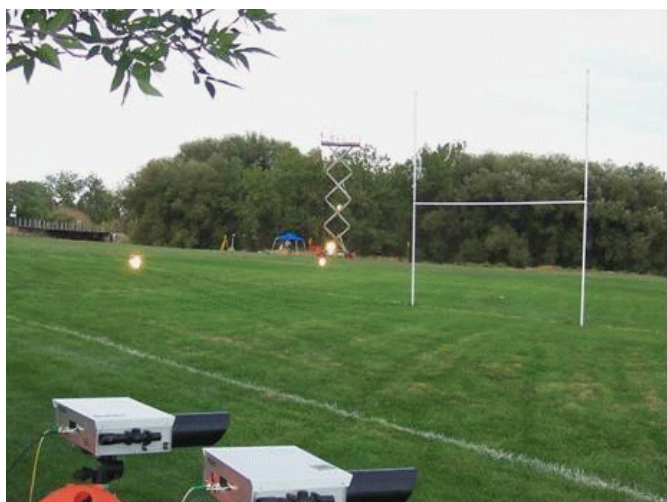
Figure 2-6. Partial Picture of the VRPM Configuration Used at the Site.
