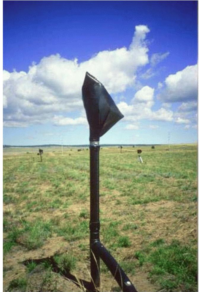
**Figure 2-1. Passive Vent Sealed During the HRPm Surveys.**
