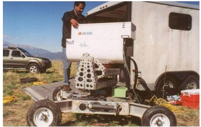
**Figure 1-4. OP-FTIR Instrument/Scanner.**
