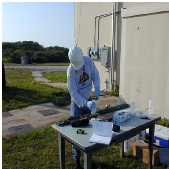
FIGURE G-3. A soil sample being collected from along the length of the core into a bottle containing methanol.
