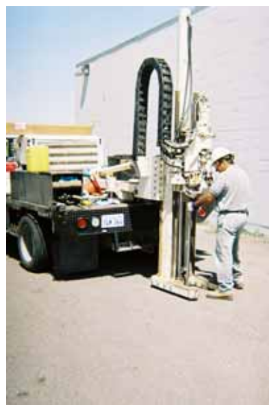
Figure 3-2. Large Direct-Push Rig
