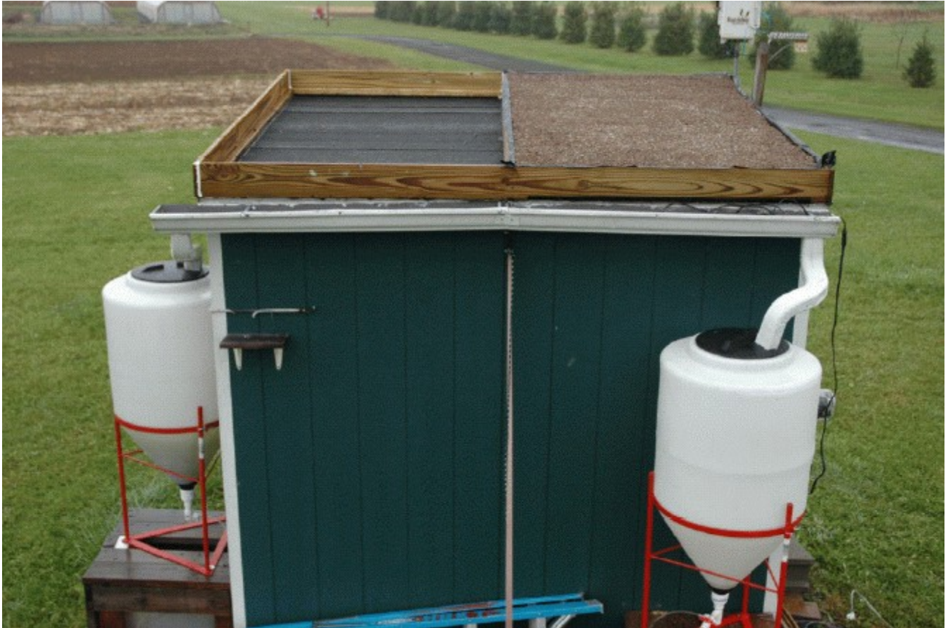
Figure A-5. One flat asphalt roof divided in half with one half filled with media and the other half sealed to detain stormwater
