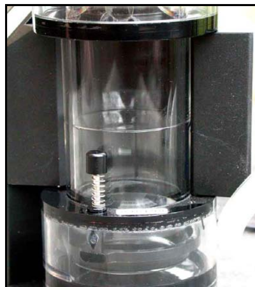
Figure 5: Soap bubble moving up the chamber. Make sure it reaches the top freely before starting measurements.
