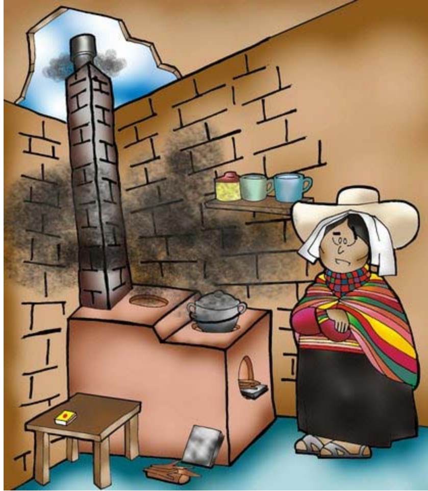
Graphic illustration depicting the smoke that is released into the room when one hole of the stove is left uncovered
