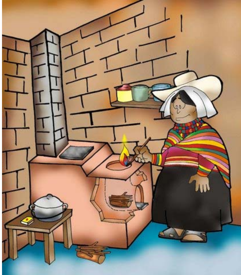
Graphic illustration demonstrating proper use of a small amount of firewood at a time in an Inkawasina improved stove
