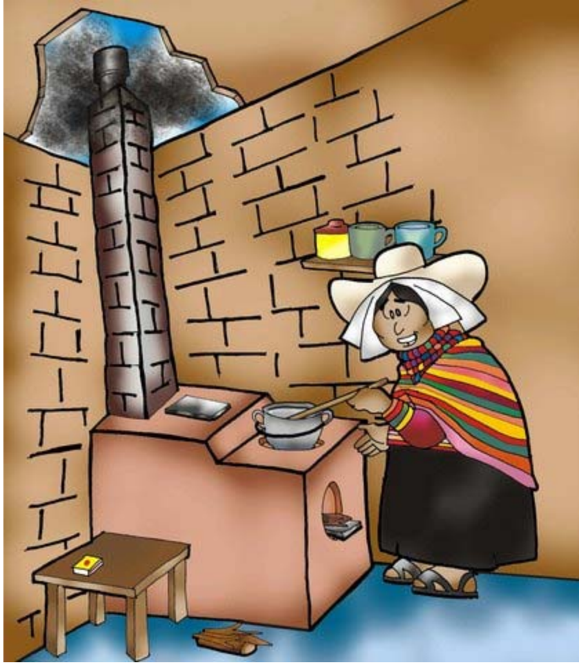
Graphic illustration depicting the proper release of smoke outside the house through the chimney when the second stove hole is properly covered
