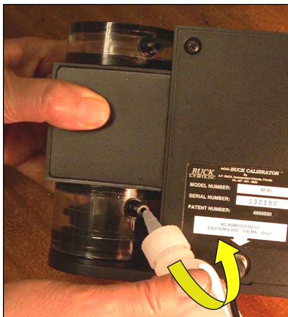
Figure 1: Place a few drops of soap solution into the bubble chamber through the lower opening.
