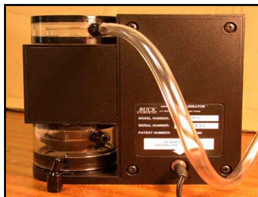
Figure 3: Tube to cyclone connects to upper outlet of calibrator.
