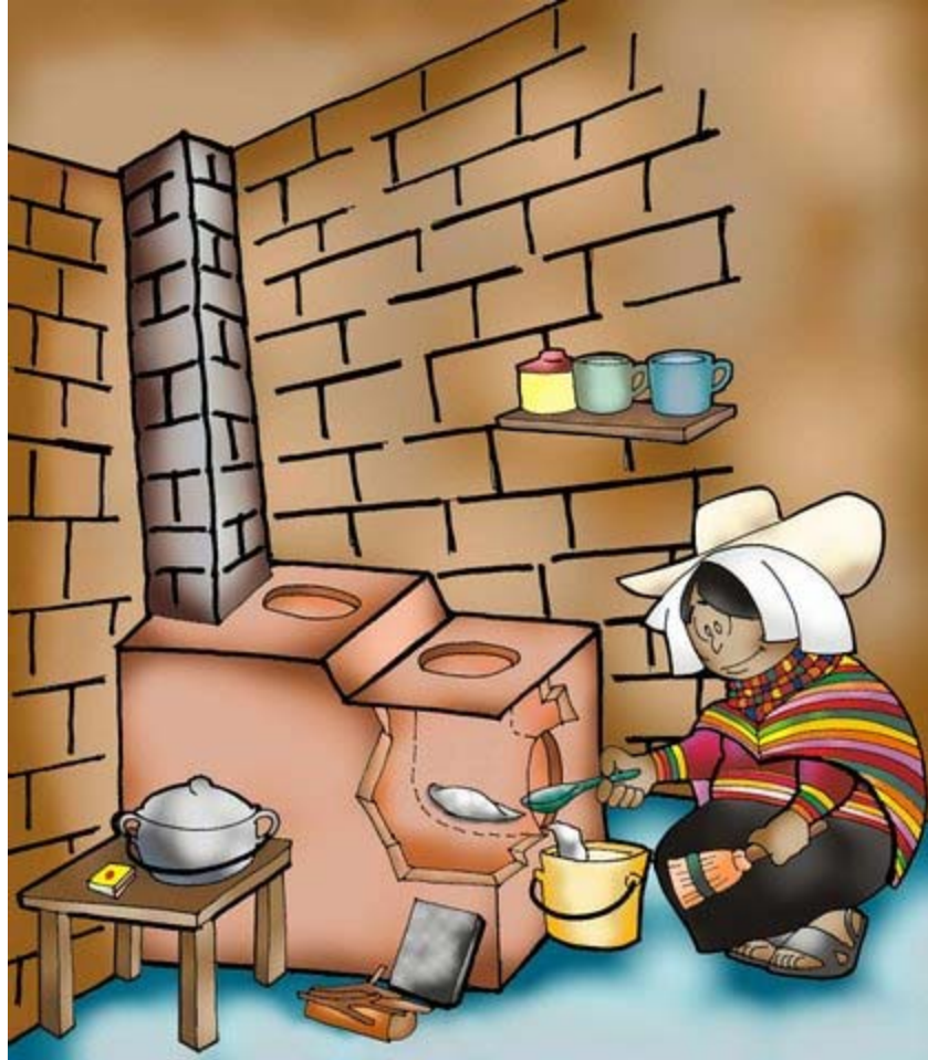
Graphic illustration demonstrating proper regular ash removal from the combustion chamber of the stove
