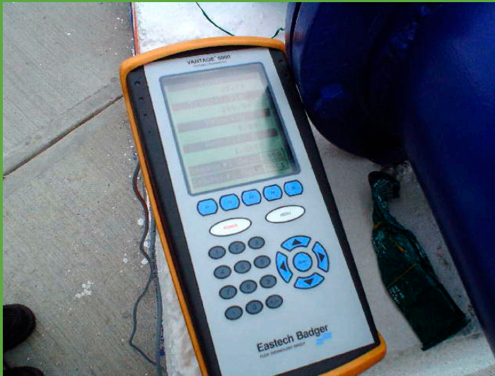
Water flow measurement equipment.
