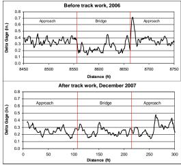
Figure 2. Gage Strength before and after Deck Replacement
