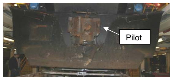
Figure 2: Front view of a locomotive pilot
