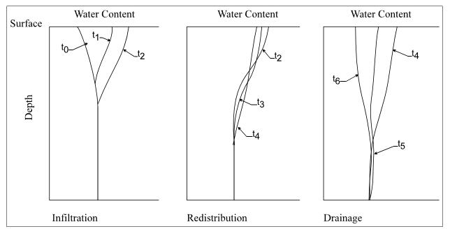
**Figure 1.** Conceptualization of water content profiles during infiltration, redistribution, and drainage (deep percolation).
