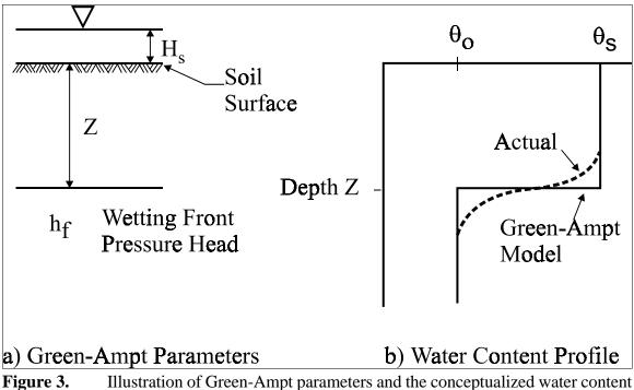
igure 3. Illustration of Green-Ampt parameters and the conceptualized water conten profile, which demonstrates the sharp wetting front.
