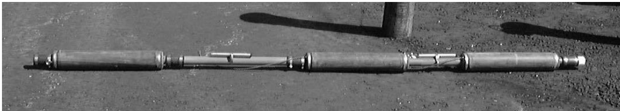
Figure 7.14 Illustration of wireless pressure transducer clamped between pneumatic packers for use in single-interval and two-interval, transient gas permeability testing in MWE wells
