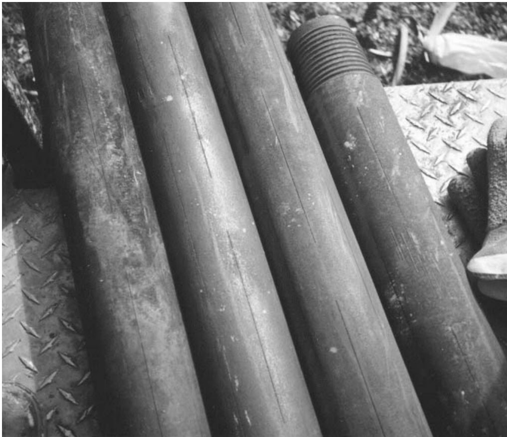
Figure 7.10 Photograph of vertically slotted 5 cm i.d. high tensile carbon steel pipe initially installed for gas permeability testing at the Picillo Farm Superfund Site.
