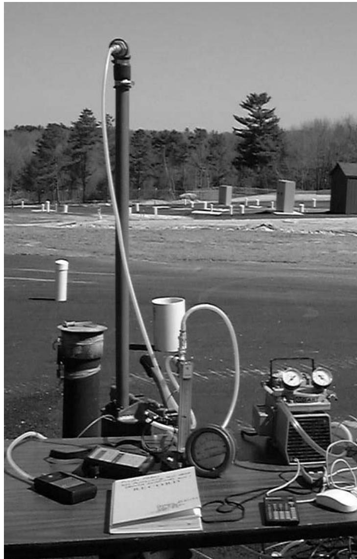
Figure 7.12 Flow, pressure, and temperature measurement at the surface during gas permeability estimation in well MWE-02
