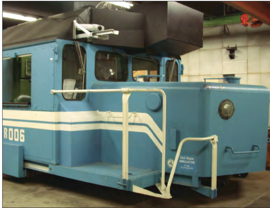
Train simulator at the Volpe Center human factors laboratory. The simulator is used to study human-factors problems in freight-railroad operations. (Photo by John K. Pollard)
