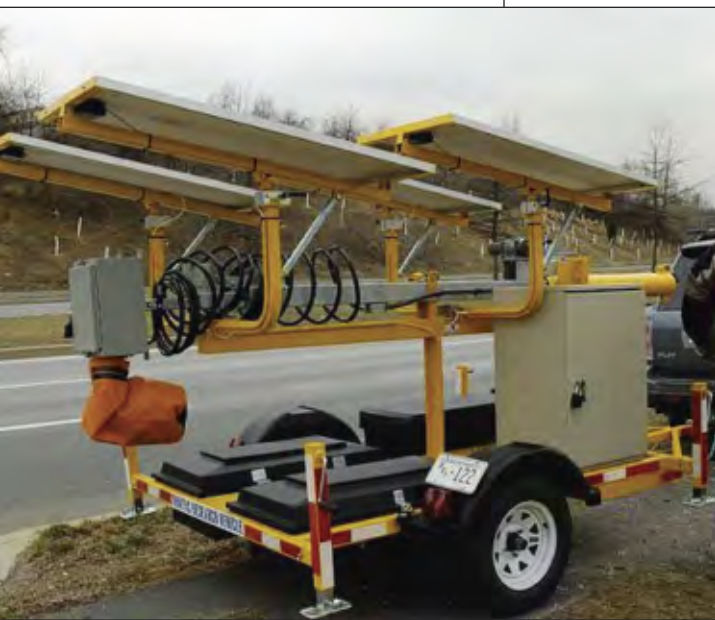
Traffic research vehicle for gathering information on vehicles approaching grade crossings; trailer design features solar charging batteries and secure tool storage. (Photo by Brian Gilleran, FRA)
