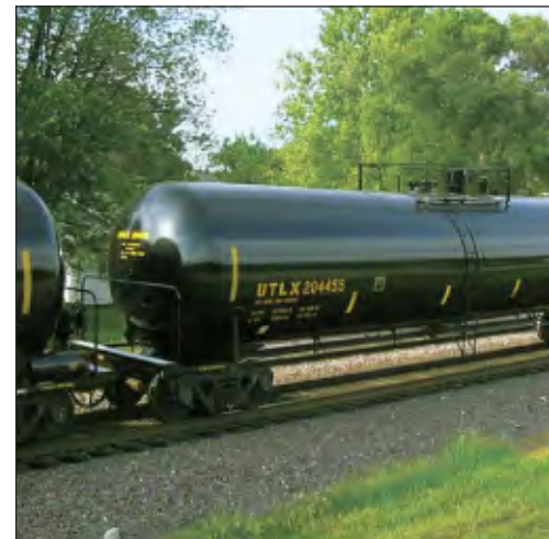
Railroad tank cars are designed to carry liquefied loads, petroleum products, liquid chemicals, and gasses. The Volpe Center supported rigorous testing of tank car impact responses as part of FRA's effort to ensure railroad tank car safety.
