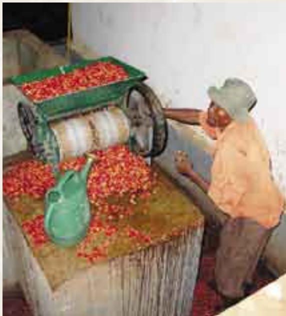
The coffee cherries are then run through a pulping machine, which removes skin and pulp that cover the bean but leaves a paper-like “parchment” over the beans.
