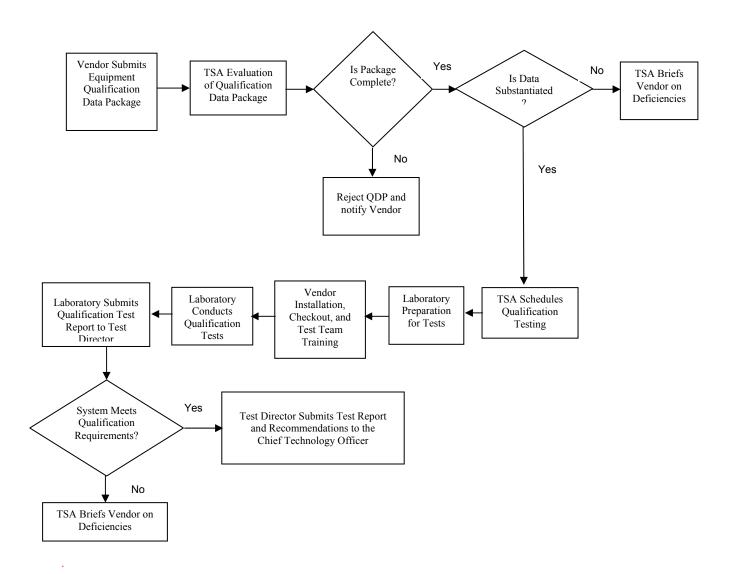
Figure 1. TSA Biometric Sub-system Qualification Test Program Flow
