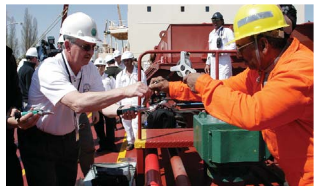
The mate places a drop of ballast water on the lens of the refractometer held by Marine Specialist, Terry Jordan, Saint Lawrence Seaway Development Corporation.
