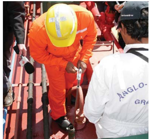
On deck, a boatswain's mate retrieves water from a ballast water tank using his sounding tape.
