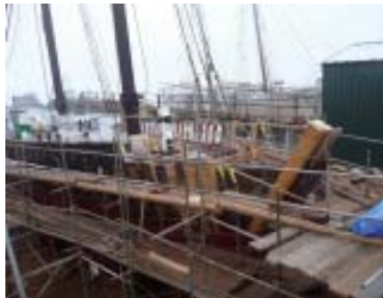
Starboard bow showing new inner stem and new frames.
