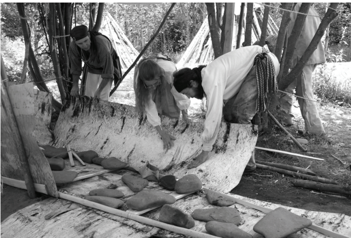
A birchbark canoe undergoing steaming of the bark and initial shaping of the bottom on the upper building bed in the Ojibwe Village.
