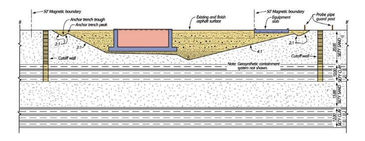
Figure 2: Cross section of CTC.
