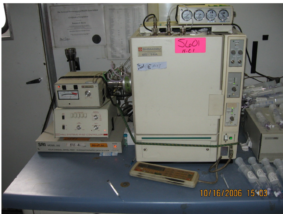
Photograph 8 – Gas chromatograph used for study.
