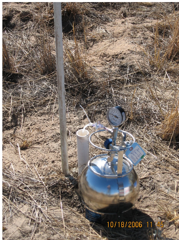
Photograph 10 – Sampling using a 6-liter SUMMA canister.
