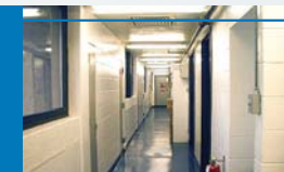
Interior Access Hall Each research module can be entered from the Interior Access Hall. This design feature helps prevent microorganisms cultured in one module from contaminating assays being run in other modules.
