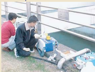
Virus in water are collected on filters
