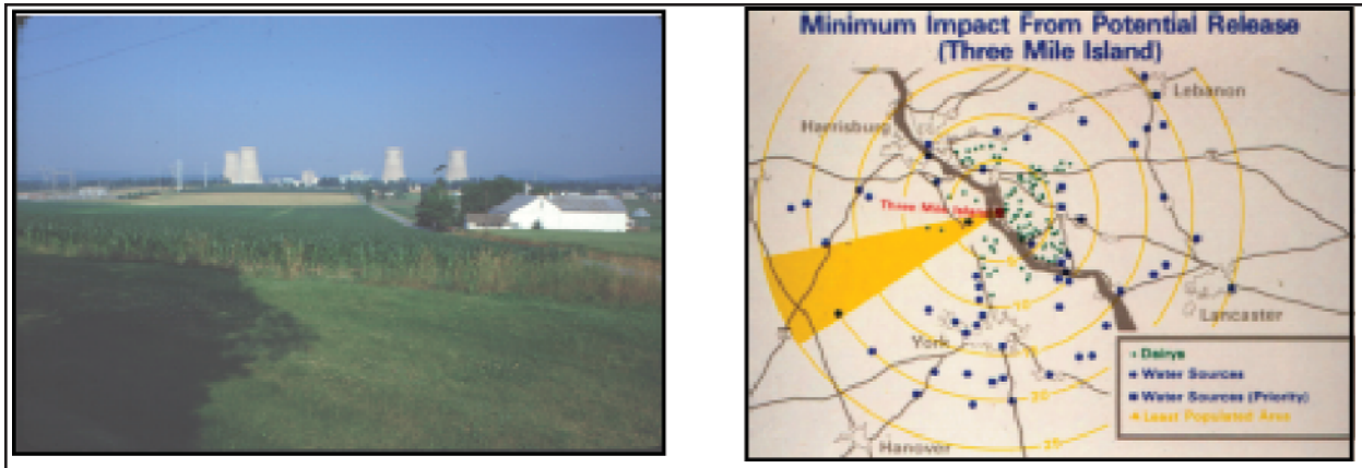
Figure 3. Three Mile Island with nearby agricultural plots and an associated map (developed from an analysis of aerial photographs) showing the distribution of dairies, water sources and potentially impacted populated areas within a 25 mile radius of the facility.
