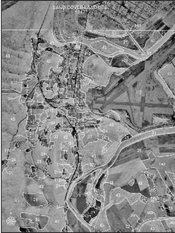
Figure 4. A land use/land cover classification of an image produced through the aerial photointerpretation process. The classification system was developed by the USGS and is a hierarchical system. For example, in the photo above, the classification divides the landscape into categories such as: 13 (industrial); 21 (cropland and pasture); 24 (farmsteads and farm-related buildings); and 43 (mixed forest).
