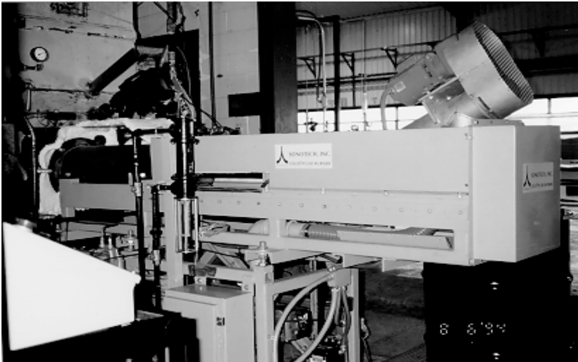
Frequency-Tunable Pulse Combustion System Installed at EPA's Research Facility
