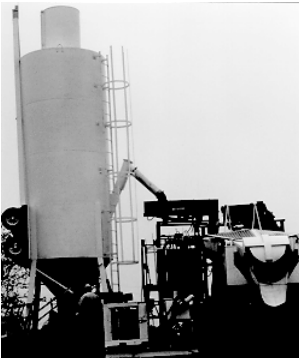
500-Ton-Per-Day MAECTITE® Processing System
