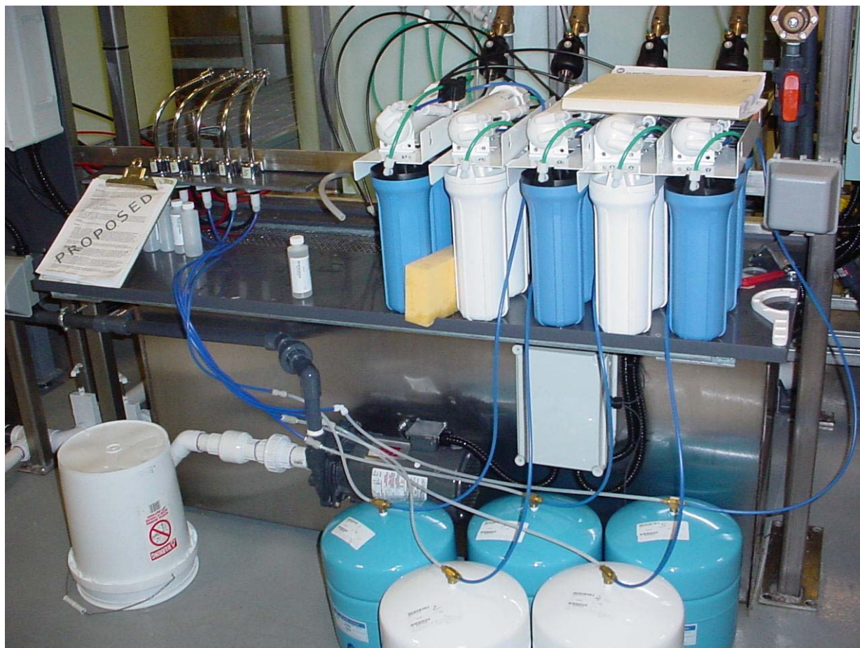
Figure 3-2. Test Units Installed on the Test Rig
