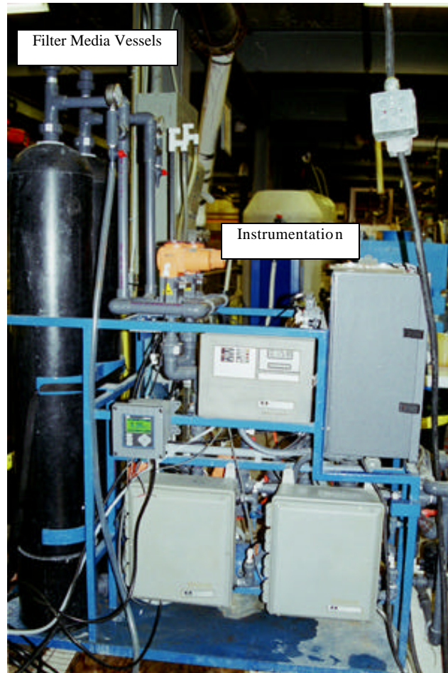
Photo 2. Side view of the Kinetico CPS100CPT Coagulation and Filtration System at SAFHL
