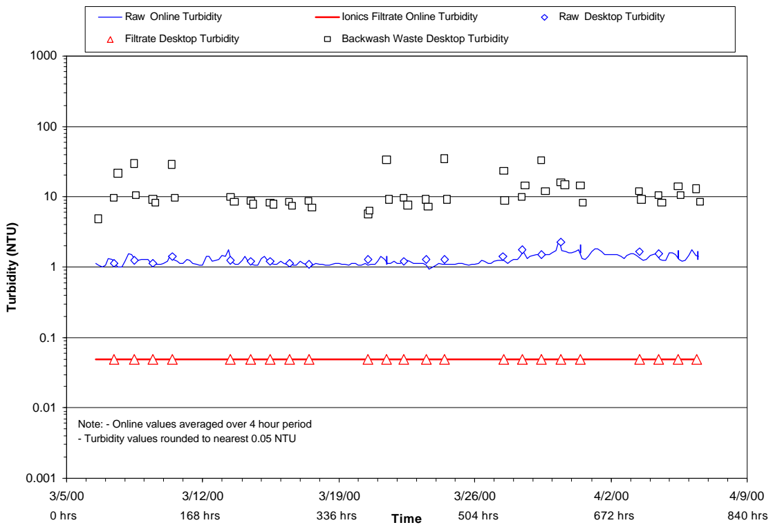
Figure 4-6. Turbidity profile for raw water and Ionics UF membrane system – Test Period 2.
