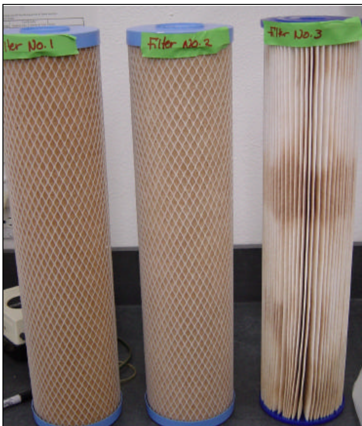
Photograph 4: Watts Premier M-15,000 RO Treatment System Pre-filters
