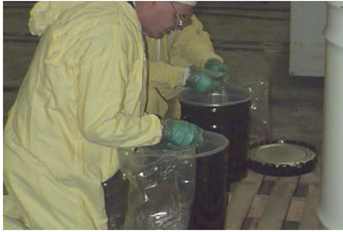
FIGURE 6: K-25 sampling personnel sift through the collected soil to remove rocks and other large debris.
