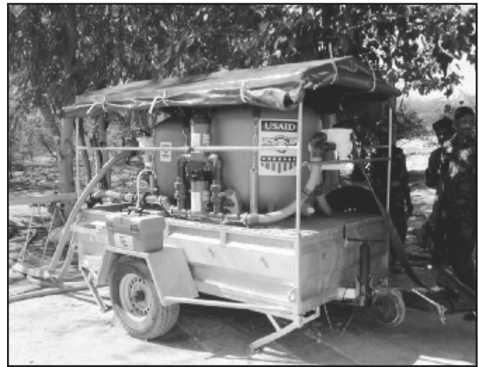
USAID/OFDA’s water purification units produced an average of 78,000 liters of water per day for families affected by the earthquake in India (photo by Michael Ernst, USAID/OFDA).
