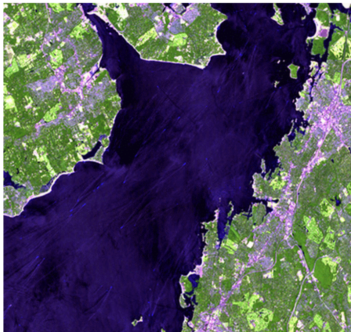
Figure 7. Landsat thematic mapper (TM) data of a coastal area, including marsh, wooded, agricultural, and urban areas.
