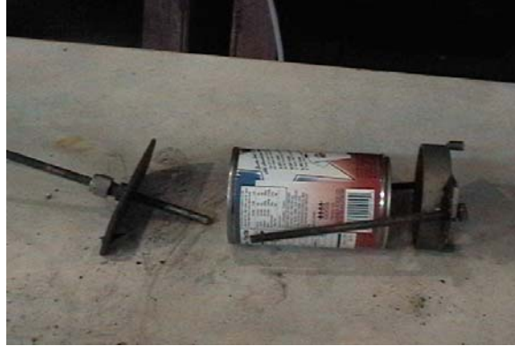
Figure 2. Thermocouple Restraining Apparatus
